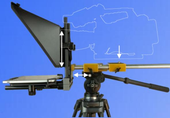
10. Mount the camera using the camera screw ensuring that the lens is in the centre of the aperture on the back of the hood. To adjust the height of the hood loosen the tube clamps, adjust to the desired height and retighten to secure. The hood and bracket assembly can be moved forwards or backwards by loosening the rod adjustment clamp. Once in the desired position retighten to secure.
