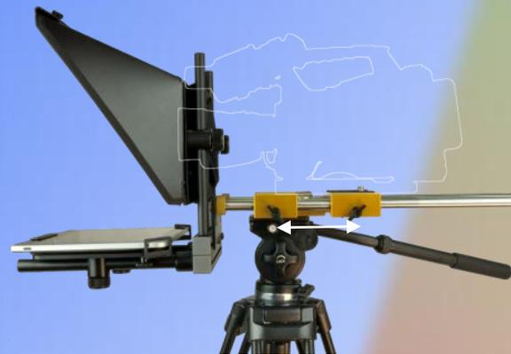
1. To balance the head with the camera mounted loosen the rod adjustment clamps, the rods will now slide freely back and forth. When you have achieved a good balance retighten the knobs, this will secure the plate in this position.
