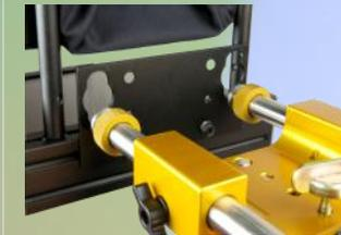
4. Mount the hood and bracket set onto the rods using the keyhole mounting holes.
