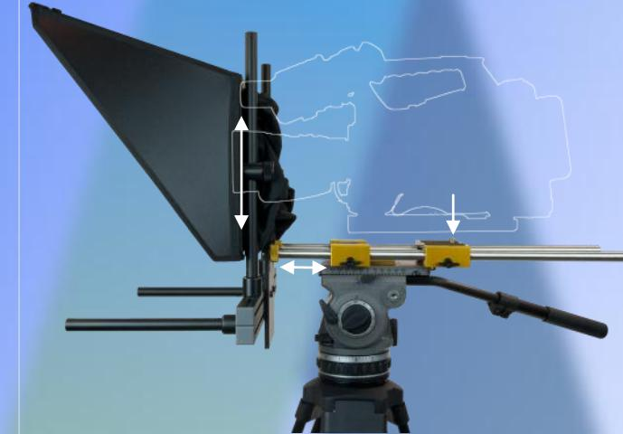
6. Mount the camera using the camera screw ensuring that the lens is in the centre of the aperture on the back of the hood. To adjust the height of the hood loosen the tube clamps, adjust to the desired height and retighten to secure. The hood and bracket assembly can be moved forwards or backwards by loosening the rod adjustment clamp, once in the desired position retighten to secure.
