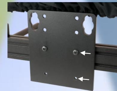
7. If needed the height of the entire bracket assembly can be adjusted by using the alternative holes in the key hole plate. Two positions are available. To move the plate remove the screws and re-fix using the alternative holes.
