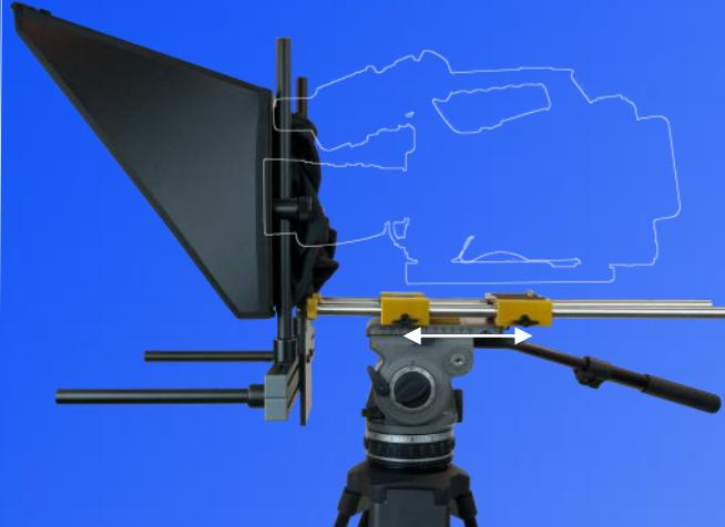
1. To balance the head with the camera mounted, loosen the rod adjustment clamps, the rods will now slide freely back and forth. When you have achieved a good balance retighten the knobs, this will secure the plate in this position.
