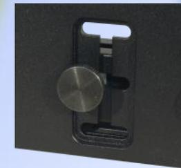
6. If needed the height of the entire bracket assembly can be adjusted by using the notched slots in the key hole plate. Three positions are available. To move the plate loosen the three knobs and move the plate to the desired height then retighten the knobs.
