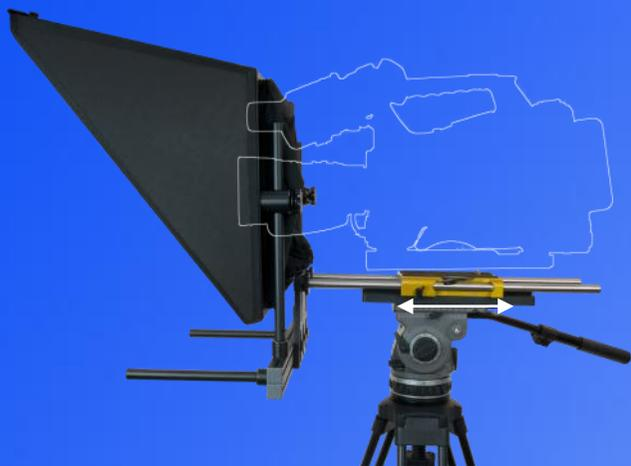
1. To balance the head with the camera mounted, slide the balance adjustment lever to the rear of the plate, the plate will now slide freely back and forth. When you have achieved a good balance slide the locking lever forward, this will lock the plate in this position.
