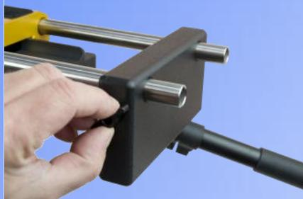
2. To lock the weight in position tighten the two clamp screws on either side. Additional weights can be added if required.
